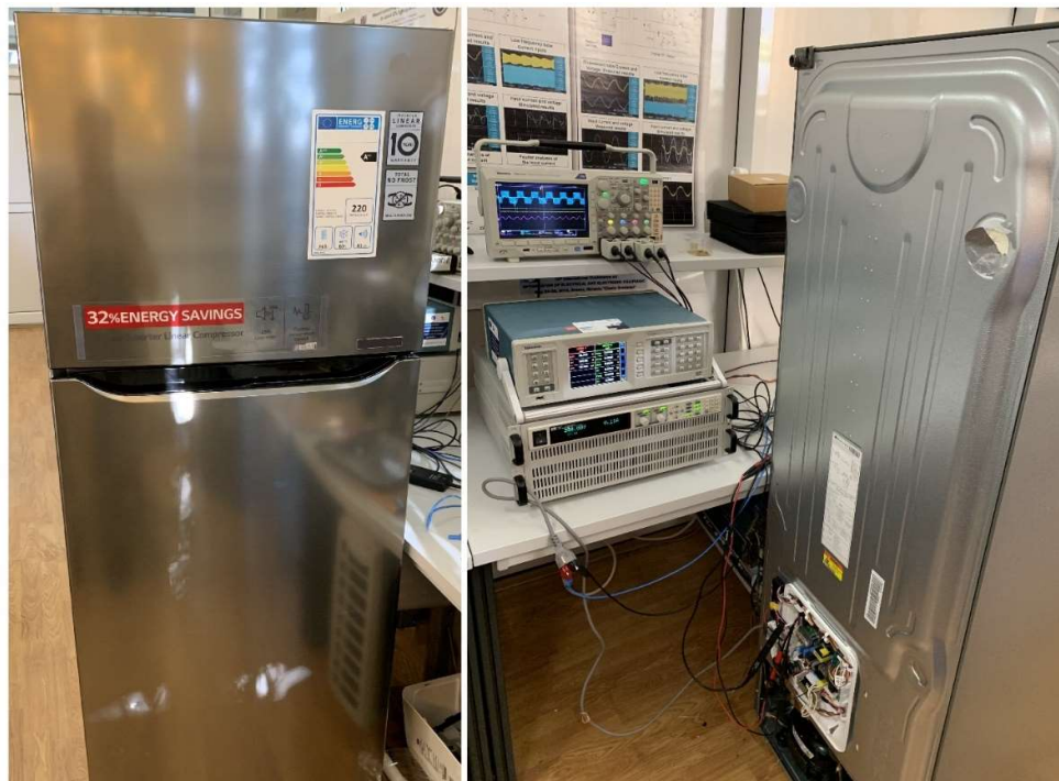
Fig. 53 Standul experimental de testare a combinei frigorifice.
