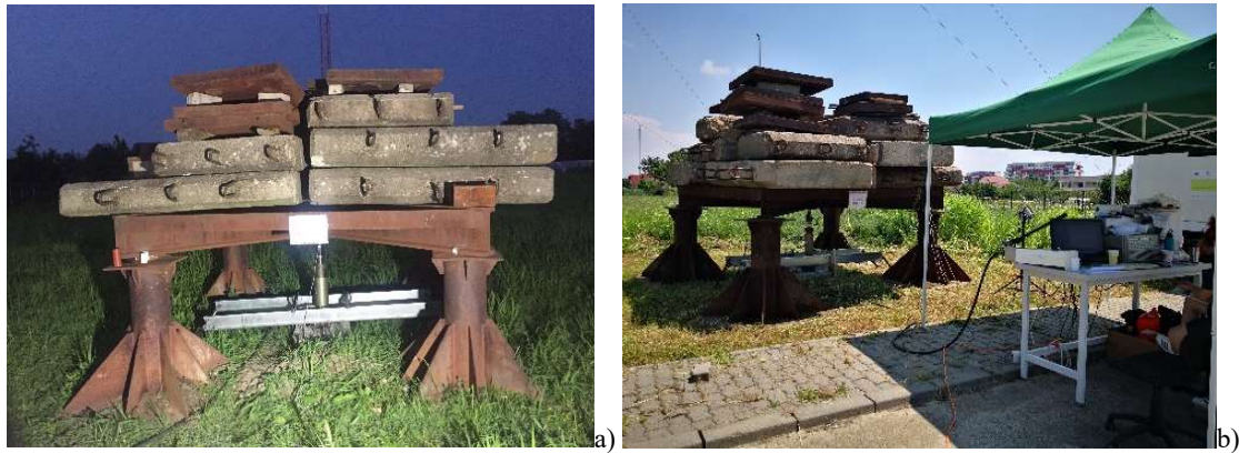
Figure 2. Ballasting of the foundation F1 (a); Loading system and data acquisition (F2) – (b).
