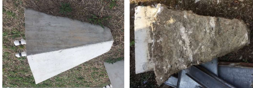
Figure 4. Shape of foundations before and after testing.
