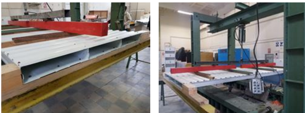
Figure 8. Overall image of the experimental setup with outer skin installed
