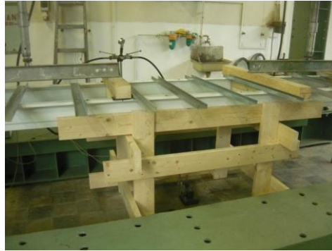
Figure 4. Mid span timber rig to prevent lateral-torsional buckling of the specimen
