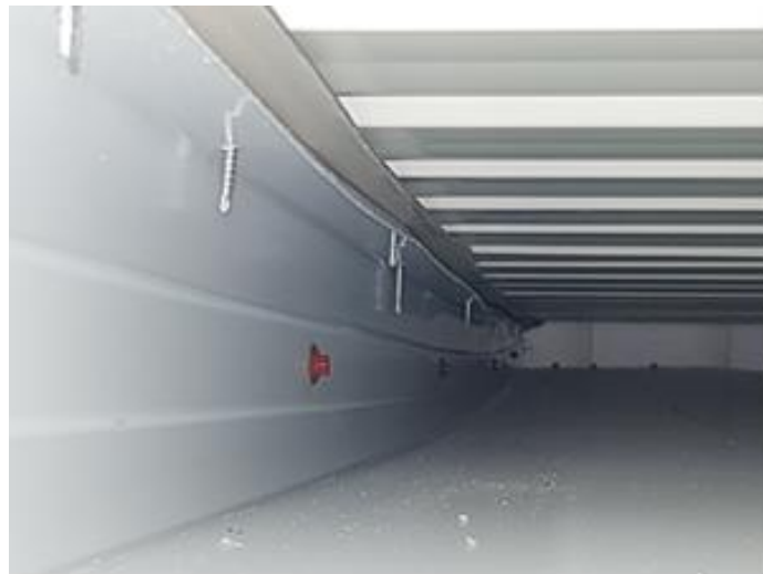
Figure 10. Local buckling of the narrow flanges in compression
