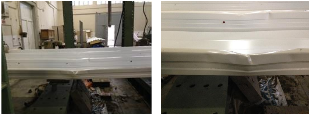
Figure 12. Failure mechanism of the tested setup
