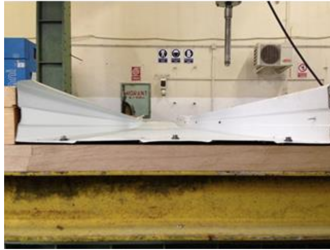
Figure 11. Uplift of wide flange central area
