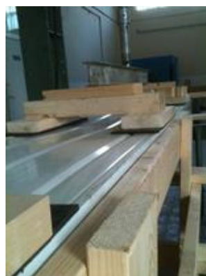
Figure 6. Smooth transmission of point load via rubber layer
