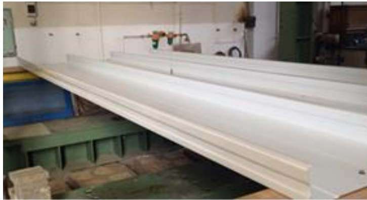
Figure 7. Arrangement using three adjacent interconnected liner tray
