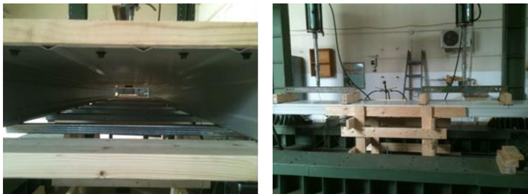
Figure 5. Experimental test setup for wind suction on cladding
