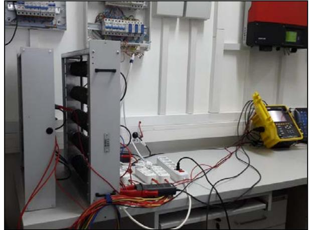
**Fig. 3.** The use of Chauvin Arnoux CA 8435 power quality analyser within the testing stand for the measurement and acquisition of power quality indicators related to the PV power plant.
