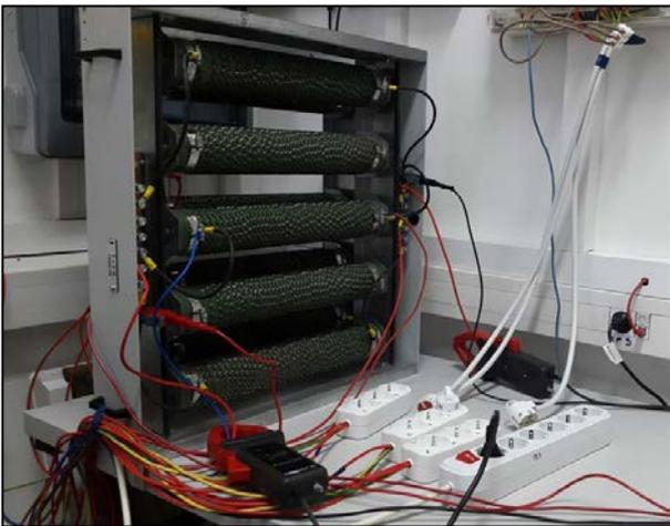
**Fig. 1.** The testing stand for the measurement and acquisition of power quality indicators related to the PV power plant.
