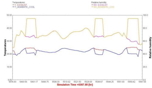
Fig. 11 Variation of the temperature and relative humidity of the air before and after the adiabatic cooling process
