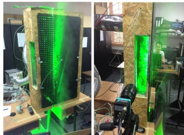
**Fig. 5.** The use of the PIV technique in order to measure air velocity profiles as a results of a metal absorber with lobed orifices – small size collector (according to [21])
